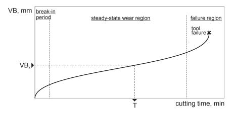
Flank wear as a function of cutting time. Tool life T is defined as the cutting time required for flank wear to reach the value of  $\rm VB_{\rm p}$
