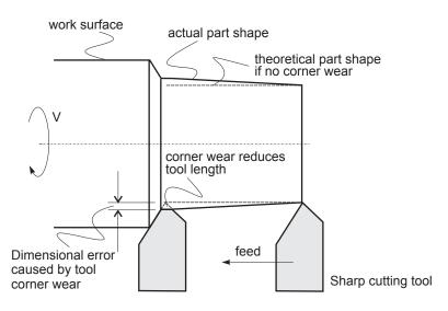
Top view showing the effect of tool corner wear on the dimensional precision in turning
