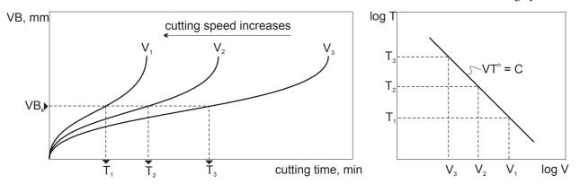
(Left) Effect of cutting speed on wear land width and tool life for three cutting speeds. (Right) Natural log-log plot of cutting speed versus tool life.
