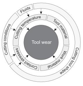
Cutting tool wear as a function of basic process parameters
