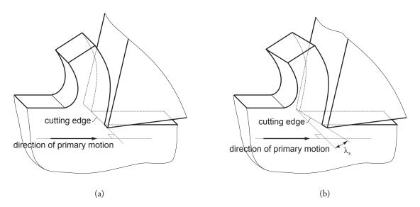
(a) Orthogonal cutting with a cutting tool set normally to the direction of primary motion; (b) Oblique cutting with a cutting tool set at the tool cutting edge inclination angle  $\lambda_s$  to the direction of primary motion.
