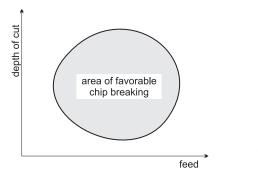
Chip map identifies the area of favourable chip formation for particular work material and cutting tool geometry
