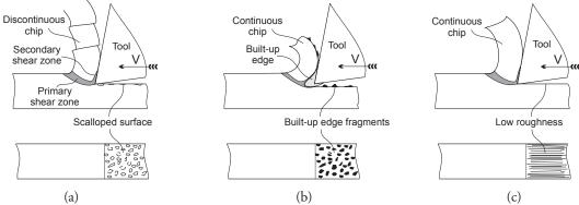
The type of chip changes with cutting speed. When cutting mild steel, the chip is discontinuous at low cutting velocity (a), forms with a built-up edge at about 0.5 m/s (b), and is continuous with well developed secondary shear zone at high velocity (c).
