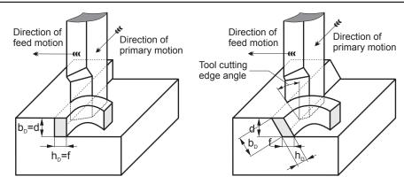
To machine a large surface, the tool must be given a feed. (*Left*) In orthogonal cutting, feed f and depth of cut d coincide with the thickness of cut  $h_D$  and width of cut  $b_D$ , respectively. (*Right*) In oblique cutting, the cutting tool edge is set at an angle (*tool cutting edge angle*) for easier chip removal.
