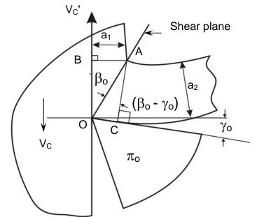
Fig. 5.9 Shear plane and shear angle in chip formation
