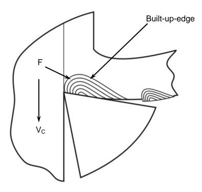
Fig. 5.11 Scheme of built-up-edge formation
