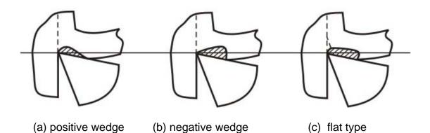
Fig. 5.12 Different forms of built-up-edge.
