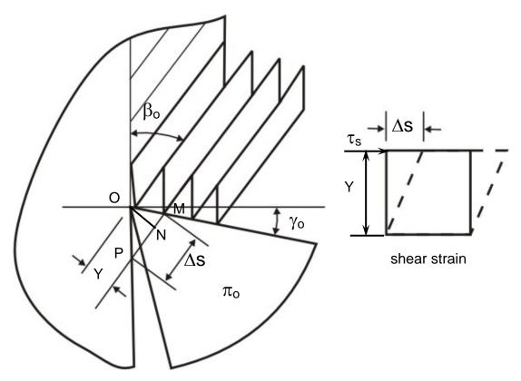
Fig. 5.10 Cutting strain in machining
