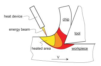
Oxyfuel torch used for thermally-assisted machining
