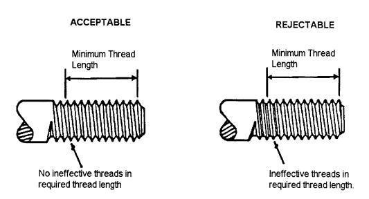
No ineffective threads within required minimum thread length. Maximum of two incomplete threads for tool runout.
