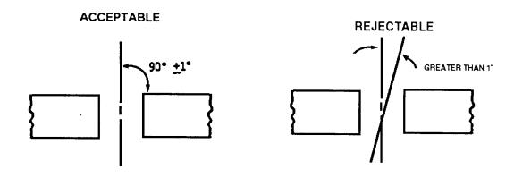
For tapped holes into materials over .125" deep or tapped through material over .125" thick, the tapped hole shall be within 1.5° of being perpendicular.
