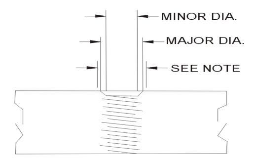
On drilled holes in flat workpieces, minimum material required to break sharp edge and deburr only, shall be removed.
