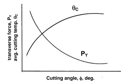
**Fig. 3.1.4** Effects of variation in cutting angle on machinability ( $\theta_c$  and  $P_y$ ) Version 2 ME III, Kharagpur
