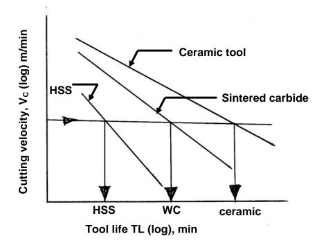
Fig. 3.1.2 Role of cutting tool material on machinability (tool life)
