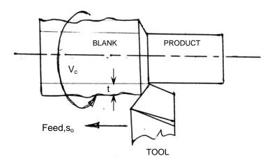
Fig. 1.4 Principle of machining (turning)
