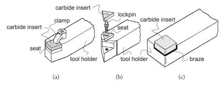
Methods of attaching carbide inserts to tool holder: (a) clamping; (b) wing lockpins; and (c) brazing
