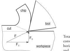
Total cutting force F is conveniently resolved into horizontal component  $F_{\rm C}$  and vertical component  $F_{\rm D}$
