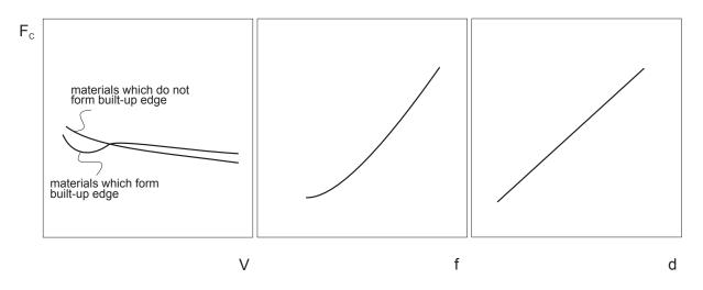
Cutting force as a function of cutting conditions
