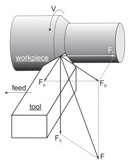
Force components in threedimensional oblique cutting
