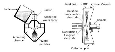
(Left) Water atomization; and (Right) Centrifugal atomization from a consumable electrode
