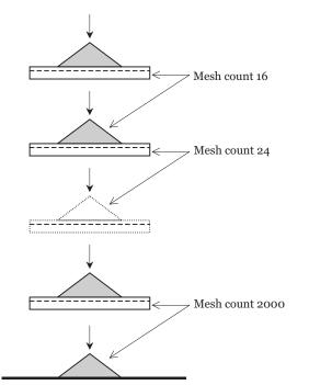
separating the powders by size is called *classification* of powders. Powders are classified by passing them through a series of screens of progressively smaller mesh size.
