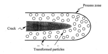
Fig. 3.3.7 The method of crack shielding by a transformation zone.
