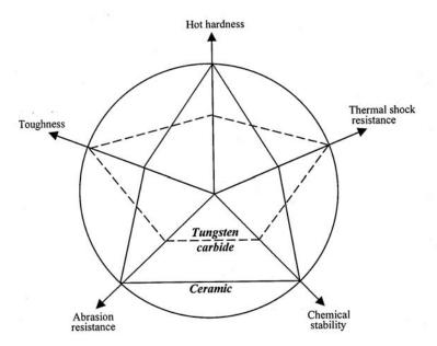
*Fig. 3.3.6* Comparison of important properties of ceramic and tungsten carbide tools
