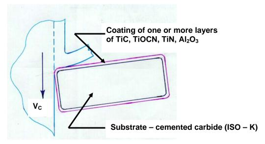
Fig. 3.3.4 Machining by coated carbide insert.
